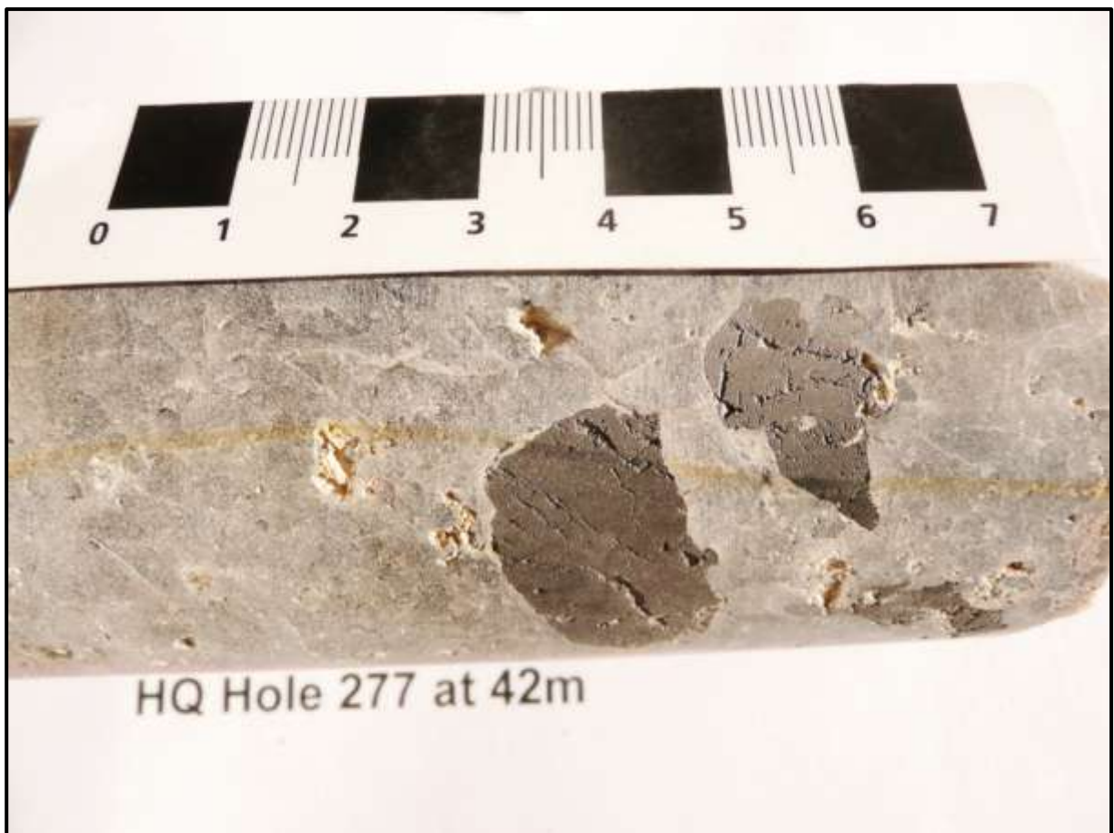
Photo 3: Hole T277C – 42m: Siliceite host rock with coarse grained tungsten mineralisation (ferberite) and white feldspar pegmatite (right). Metre interval assayed 5,405ppm WO_3 .
