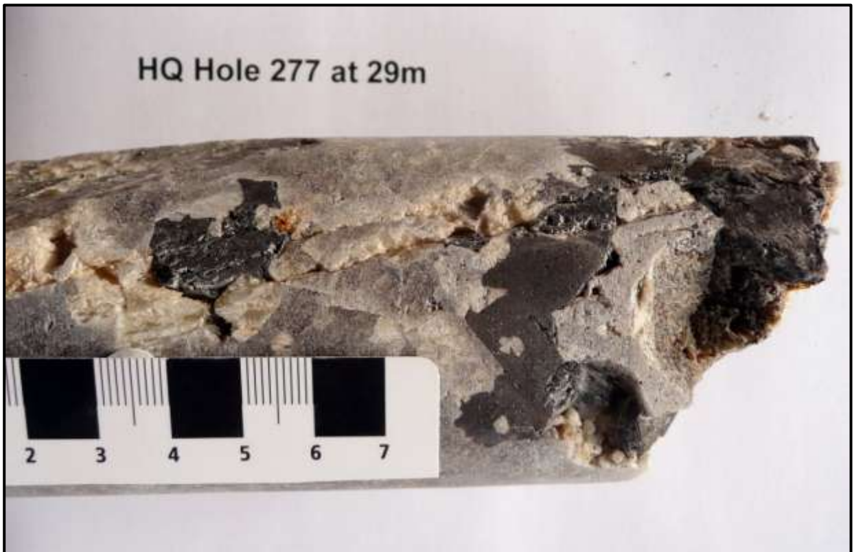
Photo 2: Hole T277C – 29m: Siliceite host rock with coarse grained tungsten (ferberite) and quartz vein. Metre interval assayed 1.23% (12,335ppm) WO_3 .
