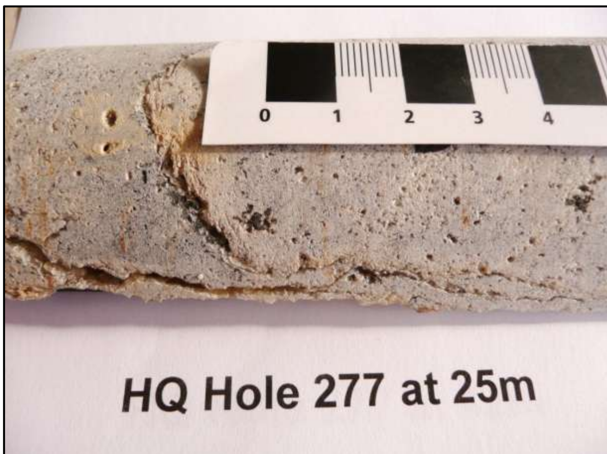
Photo 1: Hole T277C – 25m: Weathered fractured silexite with disseminated tungsten (ferberite) through silexite and on fractures. Pitting - weathered out ferberite and kaolin (muscovite). Metre interval assayed 8,618ppm WO 3 .
