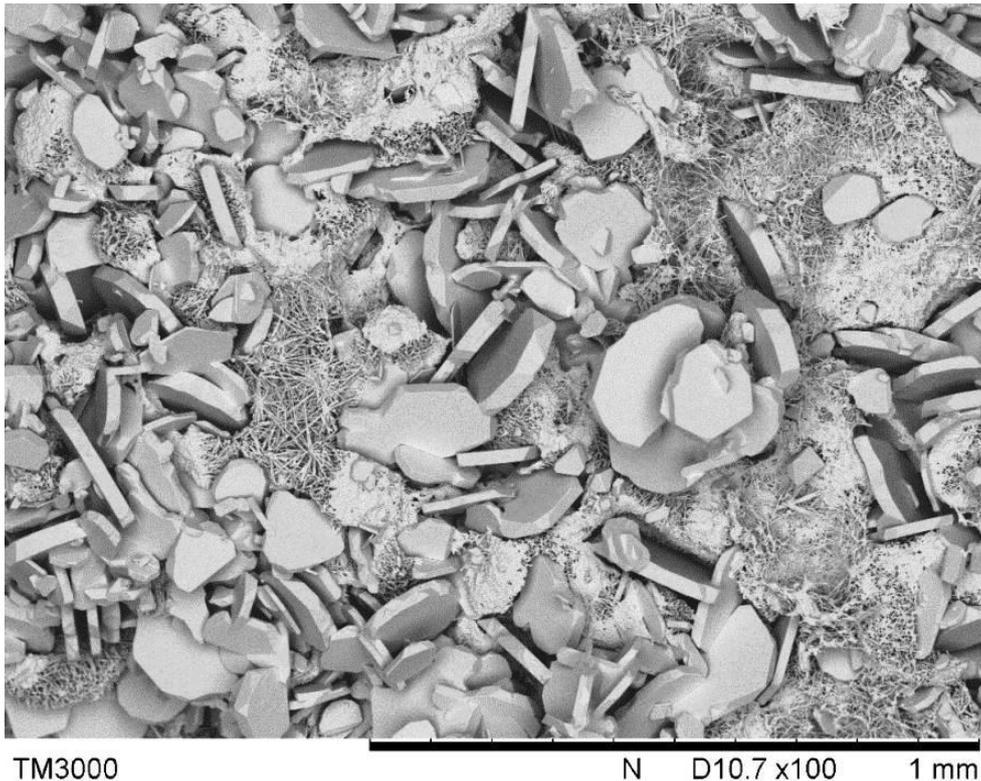
**Figure 3:** Single-crystal alumina platelets from topaz ball milled for 48 h and calcined for 2 h at 1600°C
