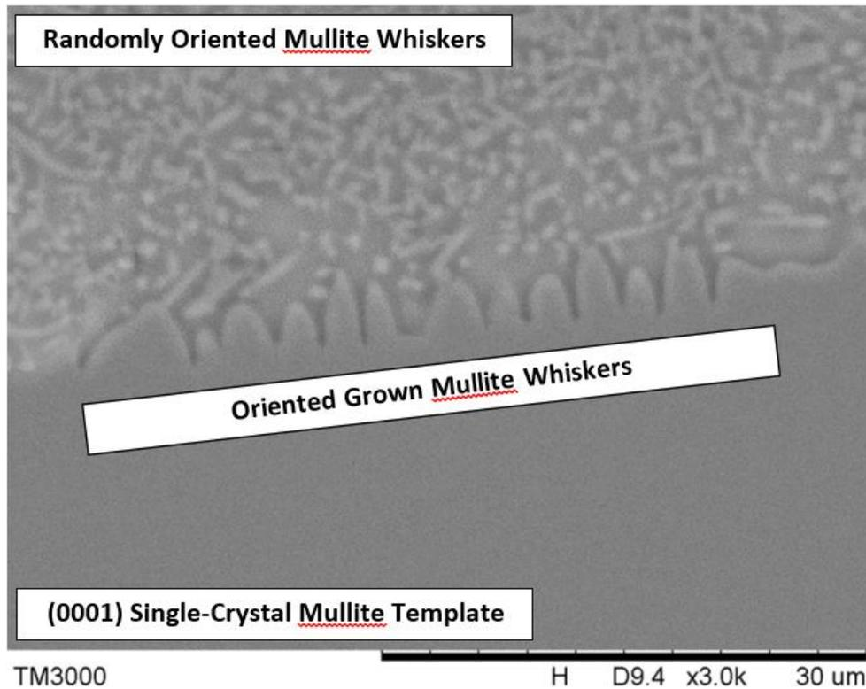
**Figure 1:** Interface between aligned (0001) single-crystal mullite and mullite from calcined topaz
